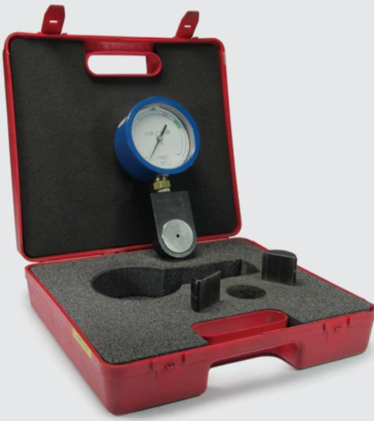
**Test gauges and manometers** are precision measuring instruments that are used to check compliance of the force developed by a tool or a hydraulic source, within just a few minutes.
