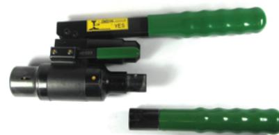
If the rail bond must be removed, the dowel will be removed using a mallet and the bushing will be removed using the bushing remover.
