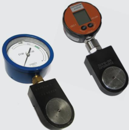
Used to check the calibration of manual and battery-operated crimping tools.
